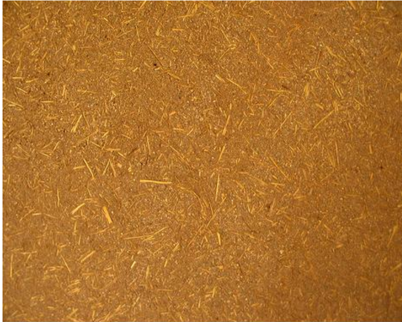
Figure 26. Earth plaster reinforced with barley straw
